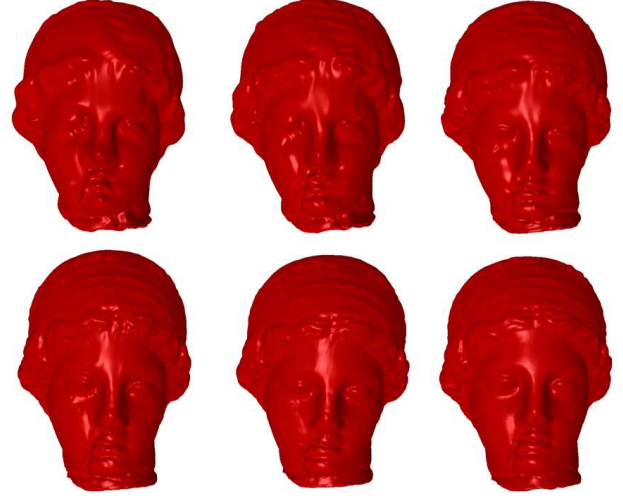
Fig. 4. Comparison of compressed meshes, from left to right: 1/16 bit/vertex, 1/8 bit/vertex, 1/4 bit/vertex, 1/2 bit/vertex, 1 bit/vertex and the original mesh.
